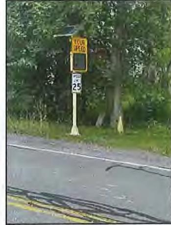
Photo 05: Speed Limit Sign with Radar Speed Display
